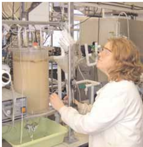
Laboratory-scale, bio-hydrogen reactor fed with wheatfeed. Source: University of Glamorgan
