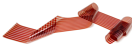
A flexible, organic bulk heterojunction solar cell
